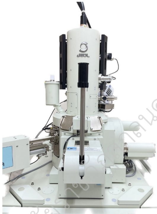
Figure 22 The Field Emission Scanning Electron Microscope-Energy Dispersive X-ray Spectroscopy (FESEM-EDS) (Ubon Ratchathani University, 2025).
