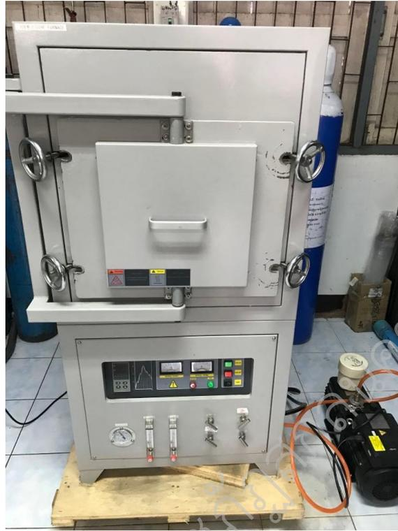
Fig. 33. High temperature furnace maximum temperature 1700 °C.
