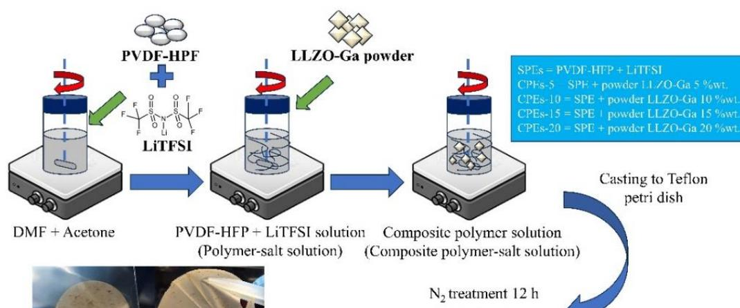
Fig. 39. Flowchart illustrating the preparation process of the CPEs.
