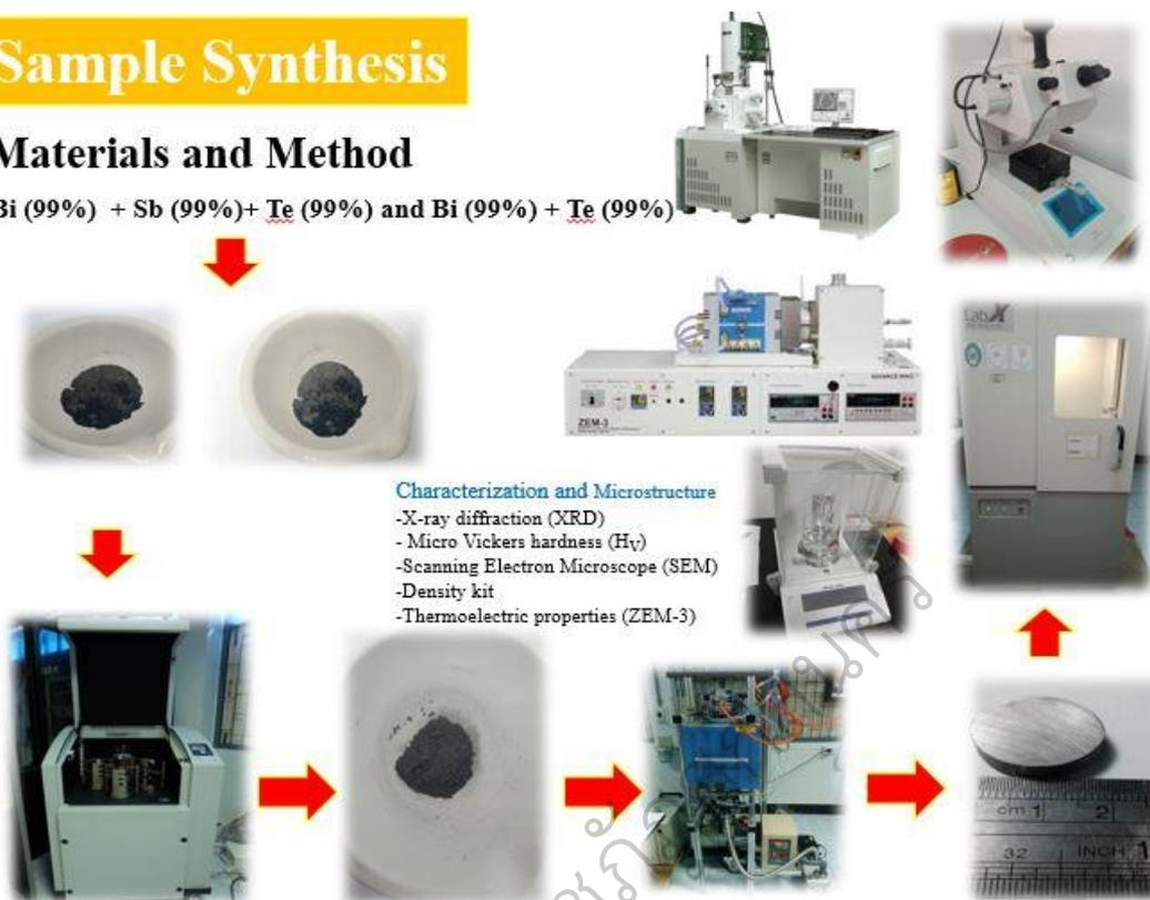
Figure 21 The sample synthesis of HP product and sintered samples
