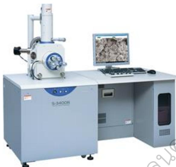
Figure 25 The SEM observations were performed on a Hitachi-S-3400N Scanning Electron Microscope at National Metal and Materials Technology Center (MTEC).
